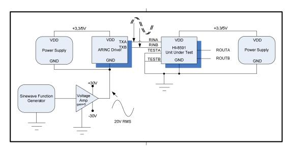
The scope plot below shows a 19.55 Volt RMS 1KHz sine wave superimposed onto the ARINC inputs. The HI-8591 still produces good ARINC digital outputs ROUTA and ROUTB. The test data is alternating 1-1 then a 0-0 pattern.
