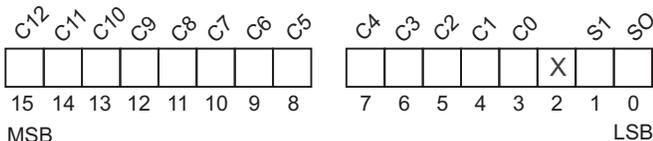
The Word Count Utility Register can be programmed to generate an interrupt on the MATCH pin when the data for the specified word count of the specified subframe is loaded into the Receive FIFO. The Word Count Utility Register can be used with any of the standard ARINC 717 data rates and all of the expanded data rates, except 8192 wps.
