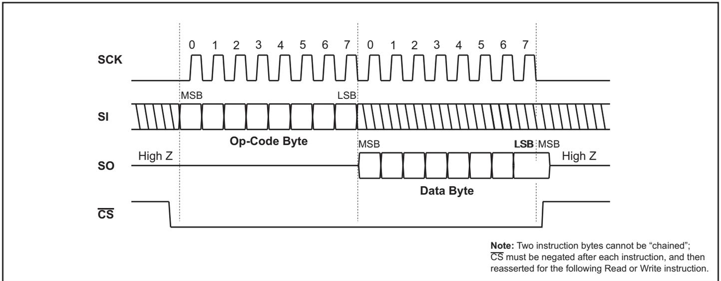
**FIGURE 3. Single-Byte Read From a Register**
