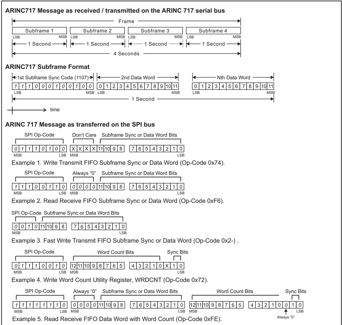
**FIGURE 5. ARINC 717 & SPI Bit Ordering**
