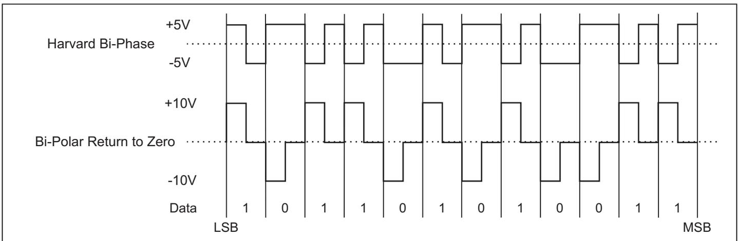
FIGURE 6. ARINC 717 HBP & BPRZ Differential Input Signal Format
