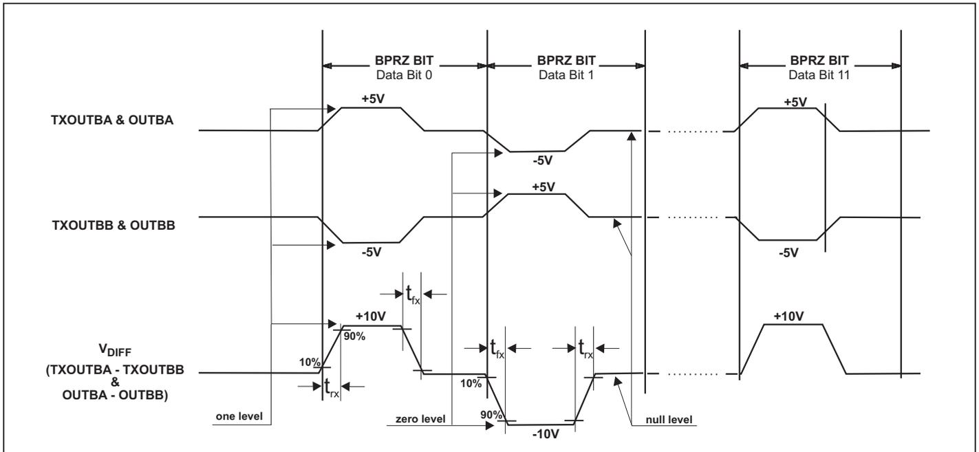
FIGURE 15. Bi-Polar Return to Zero (BPRZ) Output Waveforms
