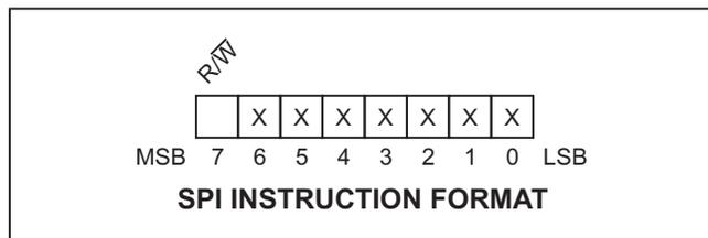
For write instructions, the most significant bit of the data word must immediately follow the instruction op code and is clocked into its register on the next rising SCK edge. Data word length varies depending on word type written: 8-bit Control & Status Register writes, 16-bit Word Count Utility Register writes and 16-bit Transmit FIFO writes.
