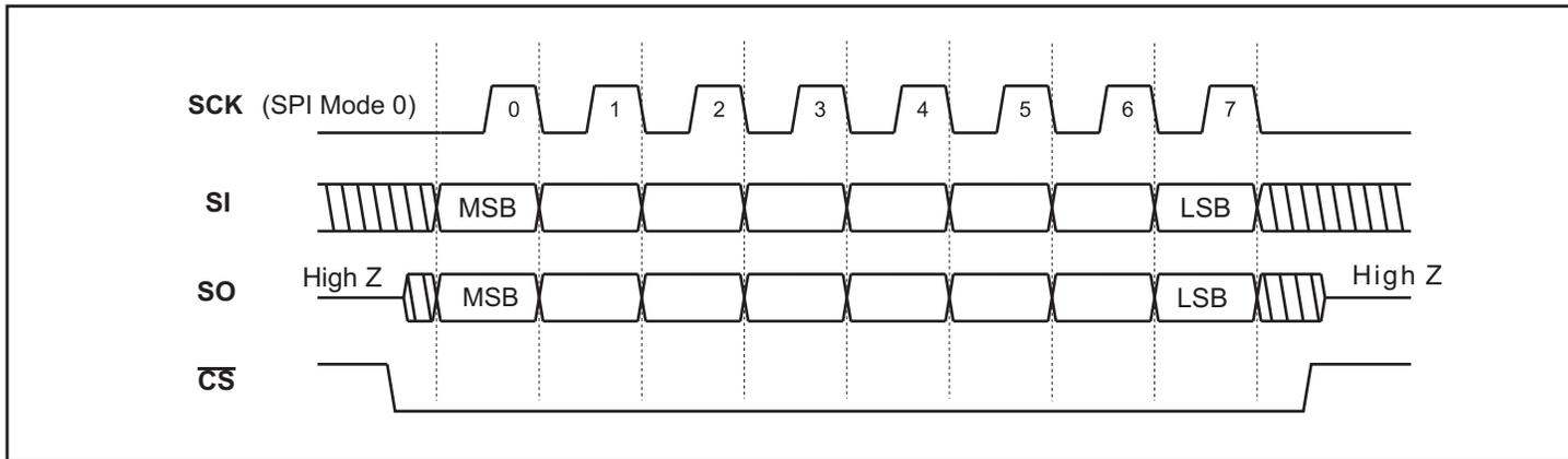
FIGURE 2. Generalized Single-Byte Transfer Using SPI Protocol Mode 0
