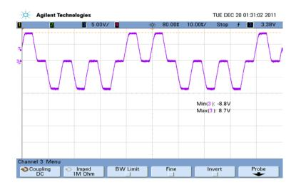
When using the HI-8190 family with the nominal power supply voltages on VLOGIC(5V), V+(15) and V-(-15V) a 20 ohm matching output resistor should be used. This assumes a 5 ohm line driver output.
