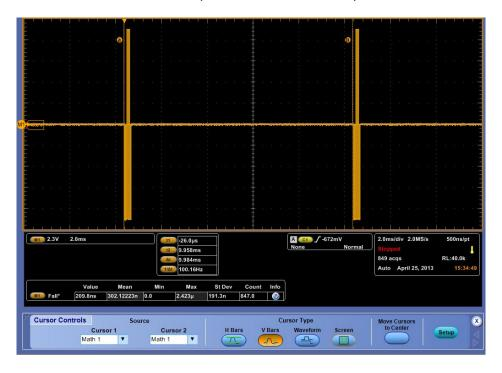
7. Remove jumpers TSTO and TST1. Use the Speed and ARINC 429 bits switch to toggle ARINC 429 output bits 9, 10 and 27 to 31, see table on the board for switch positions. Check the corresponding bit changes on the ARINC 429 output.
