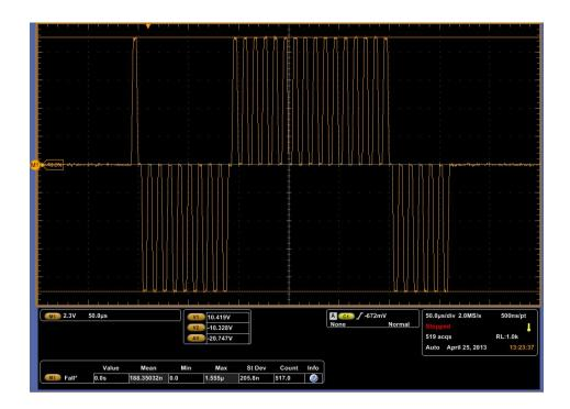
3. Now link jumper TST1 only, forcing the sensor inputs to all 1's. The output pattern for the data should be all 0's as shown below:
