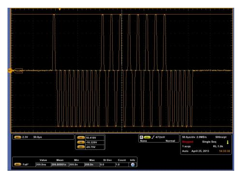
5. Replace TXENB link. Press Transmit, only one ARINC 429 word is transmitted. Change the Speed switch to '0', the waveform, should change to 12 kbps rate as shown below:
