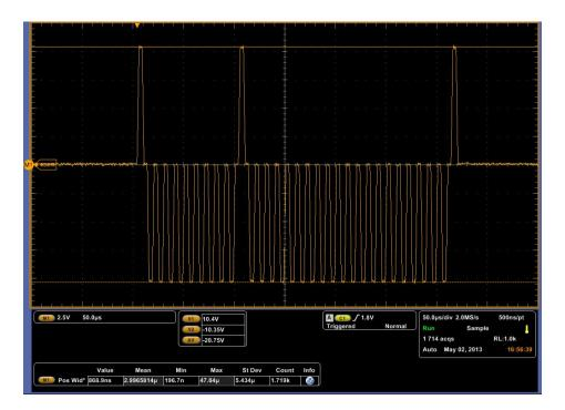
2. Set all the sensor input switches to 'ON' (GND), all the ARINC 429 data outputs (bits 11:26) should change to a '1'. This can also be checked on the connectors SENSOR OUT 0:7 and 8:15.
