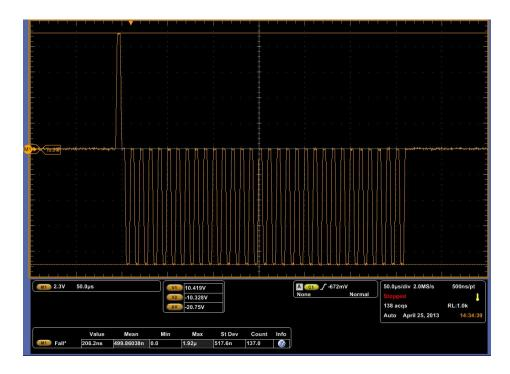
4. Now link jumper TST1 and TST0, forcing the sensor inputs to a continuously alternating 01. The output pattern for the data should be 10101010101010 be as shown below:
