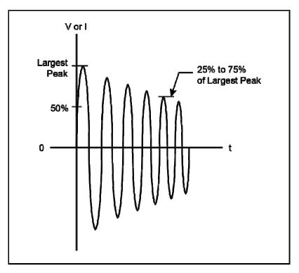
Figure 5. DO-160G Lightning Induced Transient Voltage Waveform 3. Voc = 600V, Isc = 24A, Frequency = 1MHz ± 20%.
