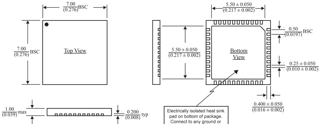
Electrically isolated heat sink pad on bottom of package. Connect to any ground or power plane for optimum thermal dissipation.
