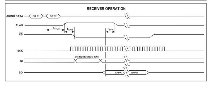
Figure 5. Timing Diagrams
