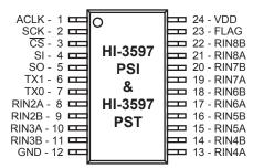
HI-3597 minimum footprint, reduced pin-out version 24 - Pin Plastic Small Outline package (SOIC)
