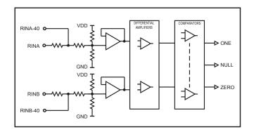
Figure 3. ARINC Receiver Input
