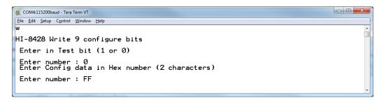
Press 'c' to read registers back to the screen and verify that the configuration reads;
