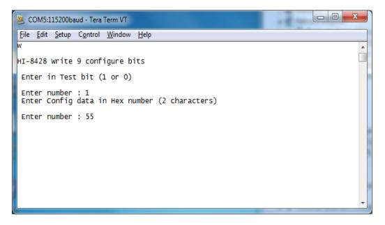
8. Press key 'c' to read configuration. The values you programmed (test bit 1, config = 0x55) should be displayed as shown in the screen below:
