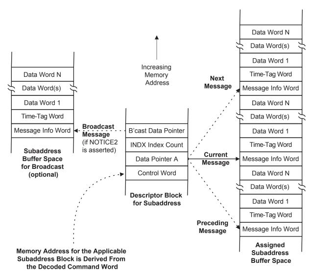
Upon successful message completion, if non-zero the INDX count in Descriptor Word 3 is decremented. If decremented result is non-zero, Data Pointer A is adjusted so next message is stored above just-completed message. If decremented INDX is zero, Data Pointer A remains static and IXEQZ interrupt occurs if enabled in Control Word.
