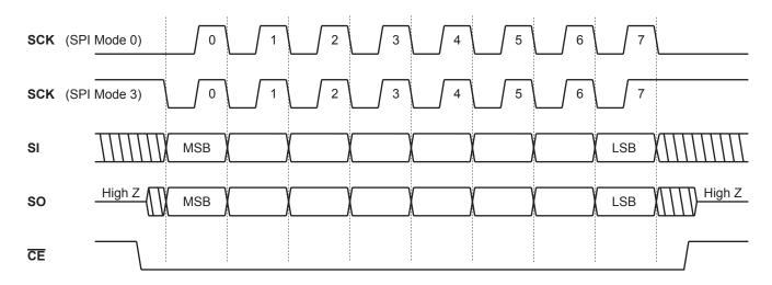
Figure 18. Generalized Single-Byte Transfer Using SPI Protocol. SCK is Shown for SPI Modes 0 and 3
