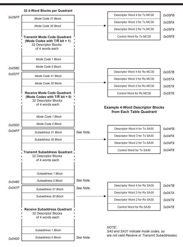
Figure 8. Address Mapping for RT Descriptor Table
