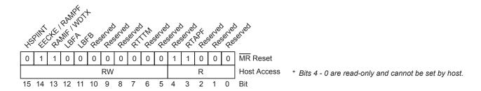
These three registers govern hardware interrupt behavior. As explained earlier, bit 2 in the Hardware Pending Interrupt Register is set whenever one or more interrupt bits are set in the RT Pending Interrupt Register. The table below first describes the common bits 15-3 in all three registers and then describes register-to-register differences for bits 2-0.
