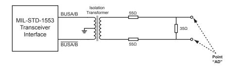
Figure 24. MIL-STD-1553 Direct Coupled Test Circuits
