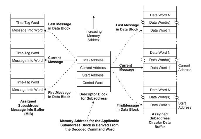
Segregated storage for data and message information simplifies host loading / offloading of buffered data.
