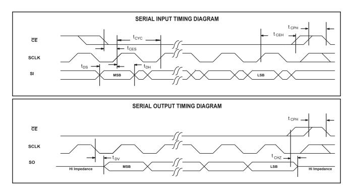
Figure 21. Host Bus Interface Timing Diagram
