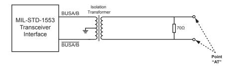
Figure 25. MIL-STD-1553 Transformer Coupled Test Circuits
