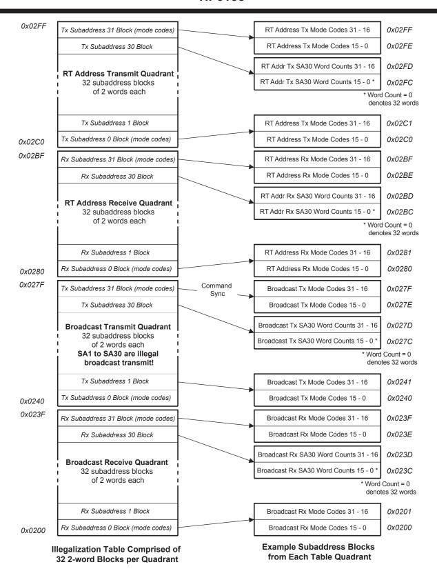
Figure 6. Address Mapping for Illegalization Table
