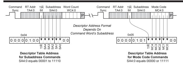
Figure 9. Deriving a Descriptor Table Control Word Address From Command Word (assumes table base address = 0x0400)
