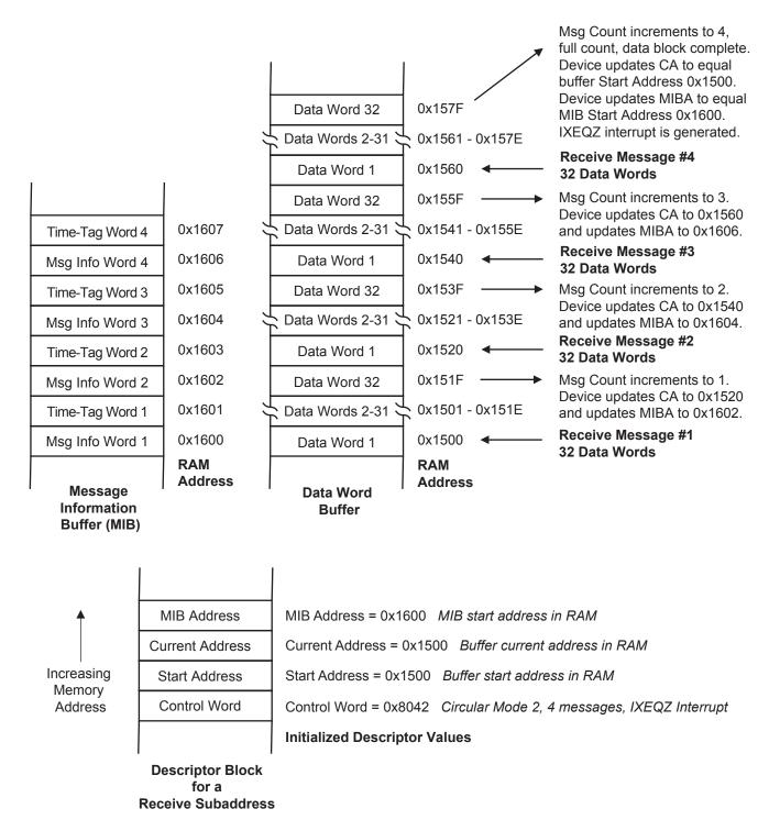
Data Block completion is based on number of messages, not Buffer Full or Buffer Empty.
