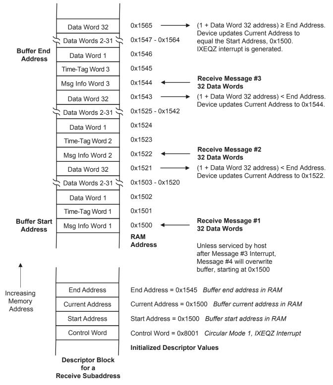
Unlike Indexed mode, Data Block completion is based on Buffer Full / Buffer Empty, not number of messages. Buffer size was purposely sized to yield remaining capacity after 2 full-count messages, to illustrate device behavior. The circular buffer should have a 33-word pad beyond its End Address to deal with buffer overrun without data loss.
