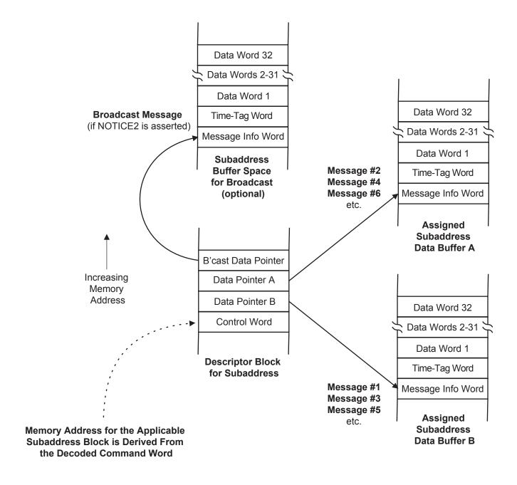
Message processing alternates between Data Buffers A and B. Upon successful message completion, the DPB bit in Descriptor Control Word is updated so next message uses other buffer. Buffers are overwritten every other message.
