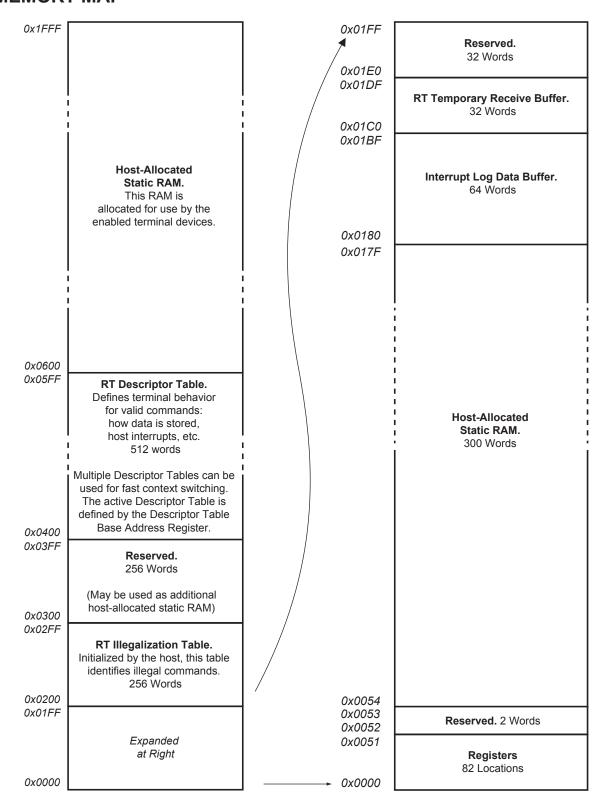
Figure 2. Address Mapping for Registers and RAM
