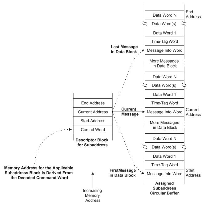
Descriptor block is initialized so Current Address equals buffer Start Address. After each successful message transaction, Current Address is adjusted to point past last data word accessed. If adjusted Current Address points past End Address, the Current Address is reinitialized to match Start Address and an optional interrupt is generated to notify host that the pre-determined data block was fully transacted.
