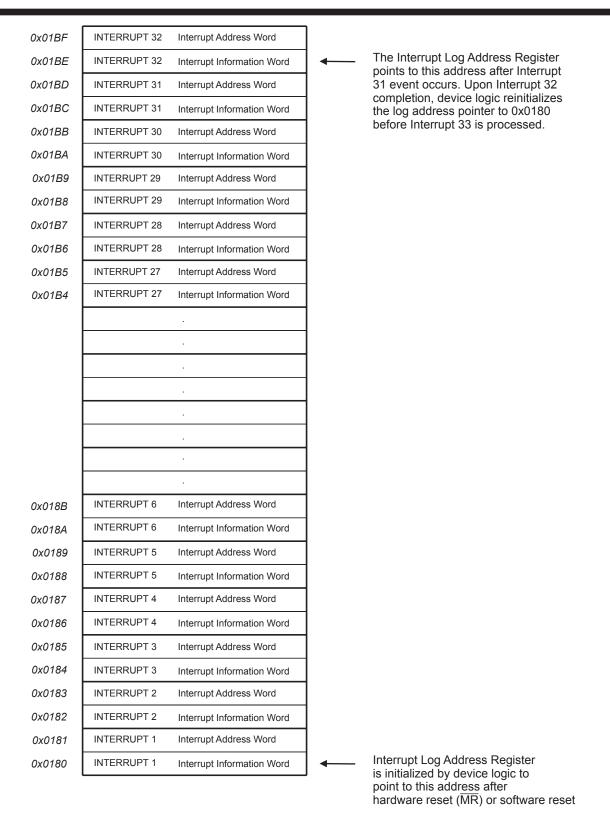
Figure 3. Fixed Address Mapping for Interrupt Log Buffer
