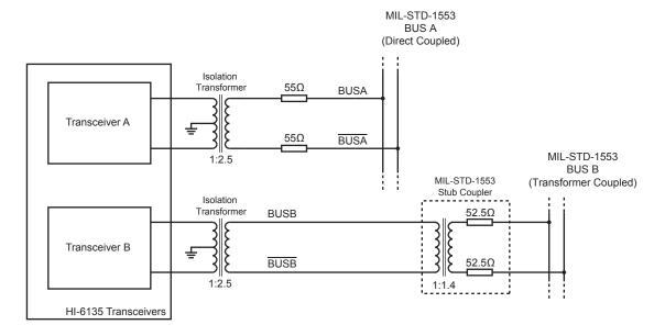
Figure 23. Bus Connection Example using HI-6135
