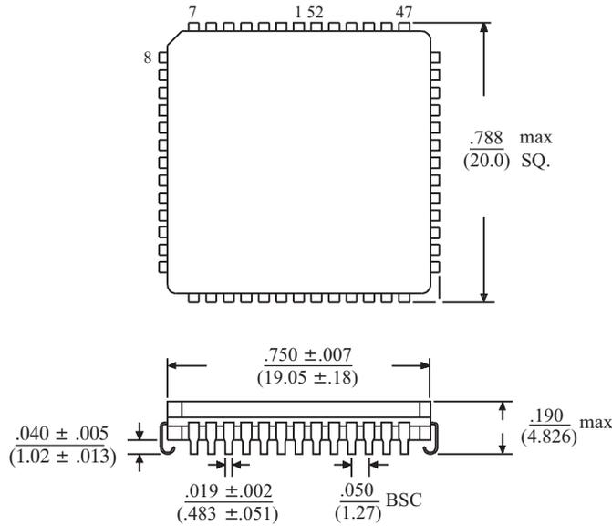
BSC = "Basic Spacing between Centers" is theoretical true position dimension and has no tolerance. (JEDEC Standard 95)
