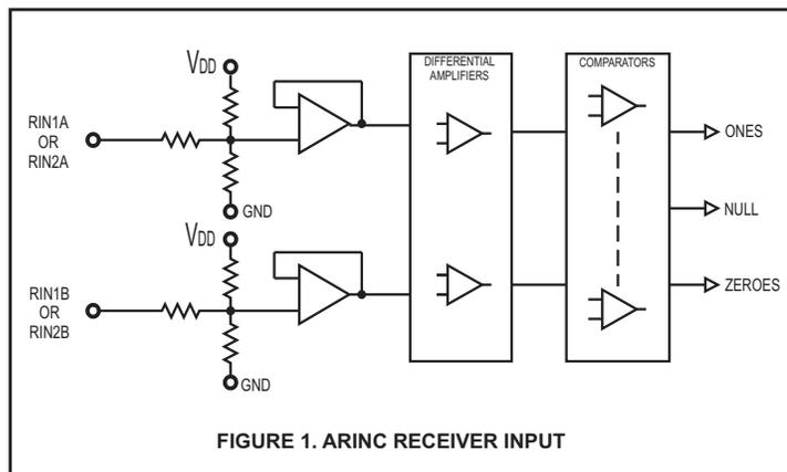
The HI-3584A guarantees recognition of these levels with a common mode Voltage with respect to GND less than ±4V for the worst case condition (3.0V supply and 13V signal level).
