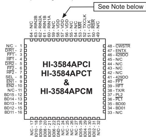
(Note: All 3 VDD pins must be connected to the same 3.3V supply)
