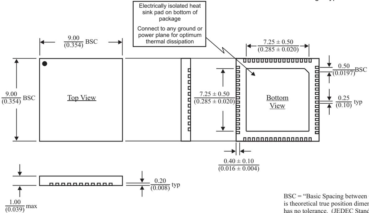
BSC = "Basic Spacing between Centers" is theoretical true position dimension and has no tolerance. (JEDEC Standard 95)
