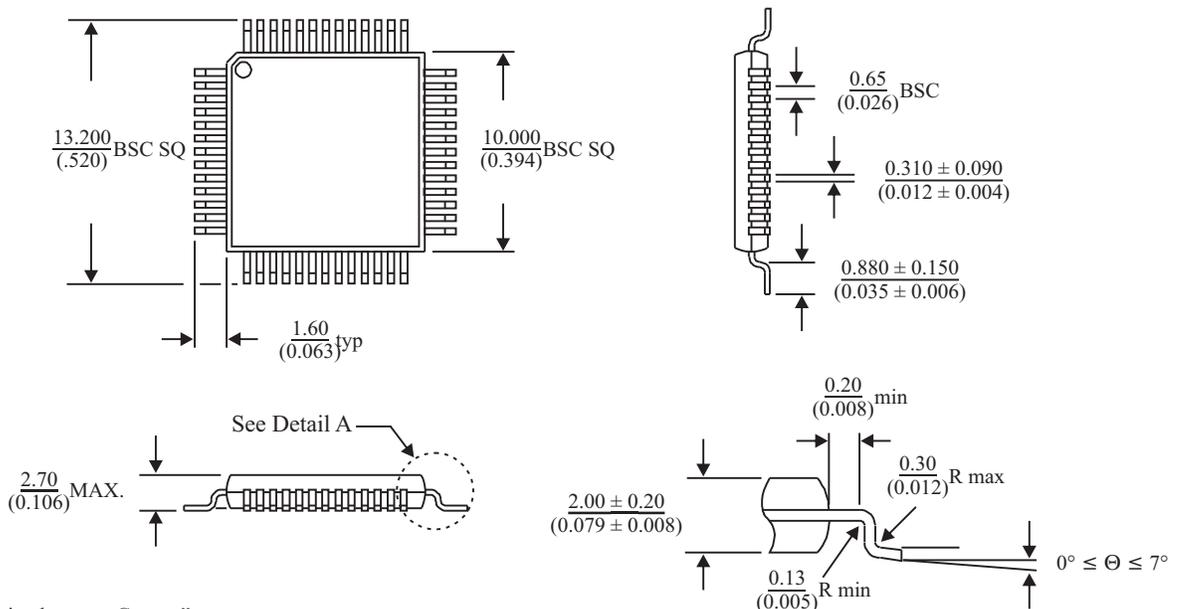
BSC = "Basic Spacing between Centers" is theoretical true position dimension and has no tolerance. (JEDEC Standard 95)
