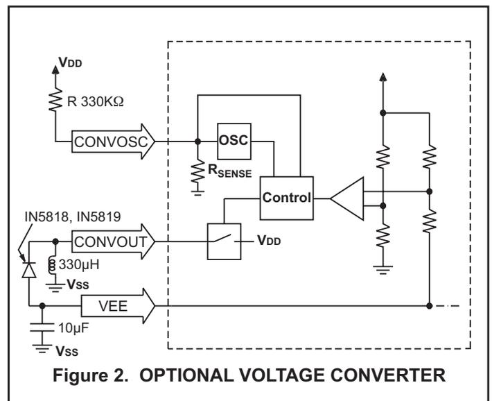
Figure 2. OPTIONAL VOLTAGE CONVERTER
