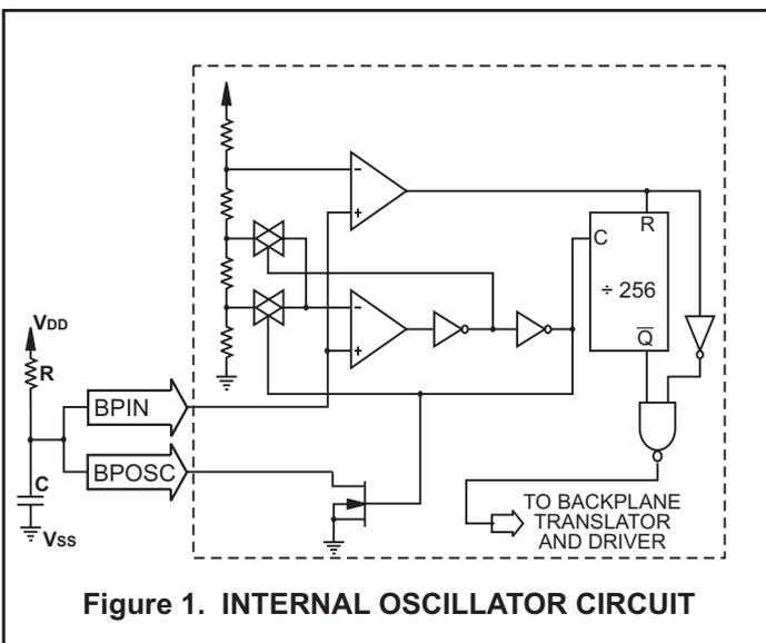
Figure 1. INTERNAL OSCILLATOR CIRCUIT
